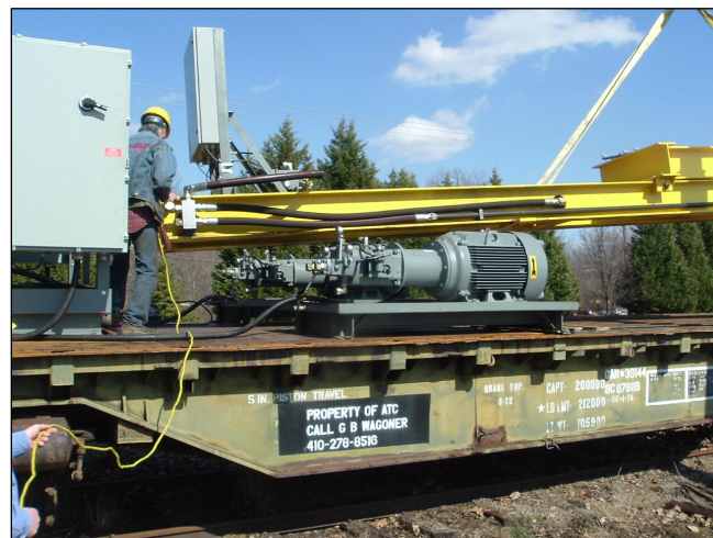
Hydraulic Rail Car Positioner to Test Sliding Ramp Foot/Vehicle Interaction
